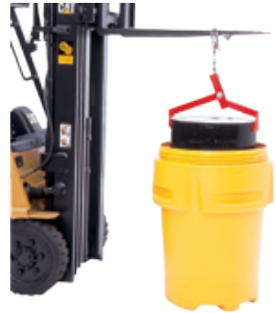
409 Drum Lifter - Securely grips 209L steel drums when loading and unloading salvage drums, Rugged, all-steel construction, Load capacity: 455 KG.
