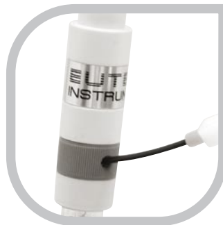
Pour in reference electrolyte with the refilling bottle (that is supplied with all electrodes)
