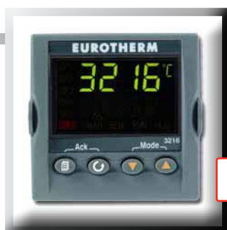
PID Control display system
